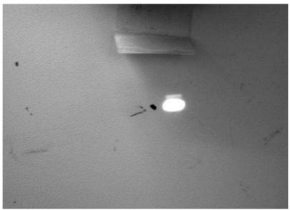
**Figure 1. BL04-MSPD:** First x-ray beam at the experimental hutch of BL04-MSPD.
