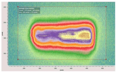
**Figure 1. BL13-XALOC:** Picture of a partly focused x-ray beam at sample position (YAG) as seen with the diffractometer's on-axis viewing system.
